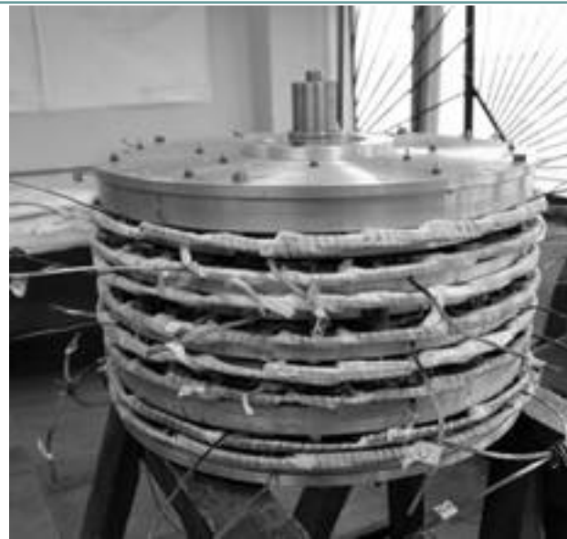
Fig. 1. Assembly process of multi-disc cryogenic motor
